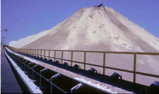
Fig 8 (a) Dry transport to a stack in a valley
