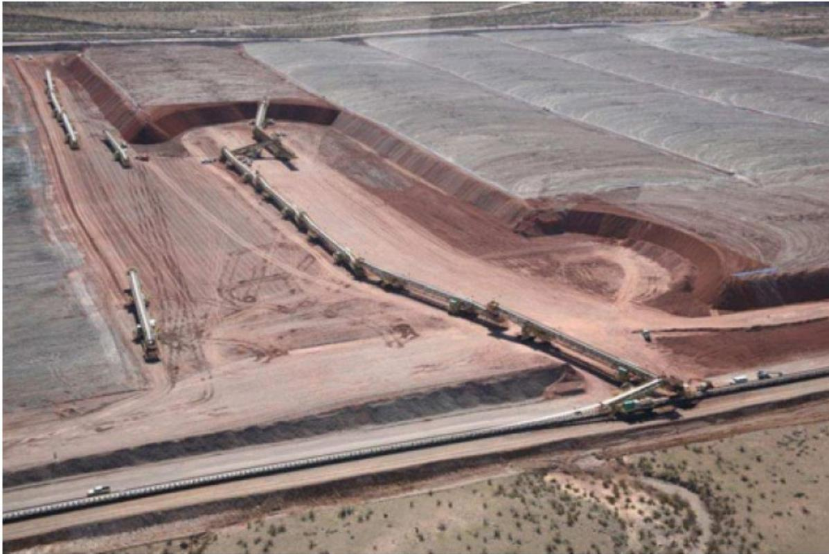
Fig 11. Self-contained movable spreader/stacker
