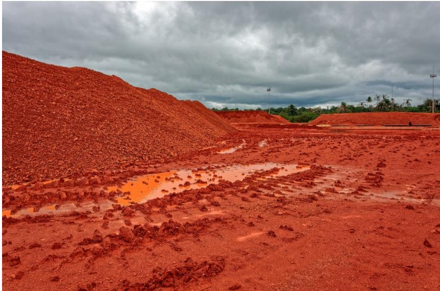
*Alumina refinery "red mud" dry stacking.*
