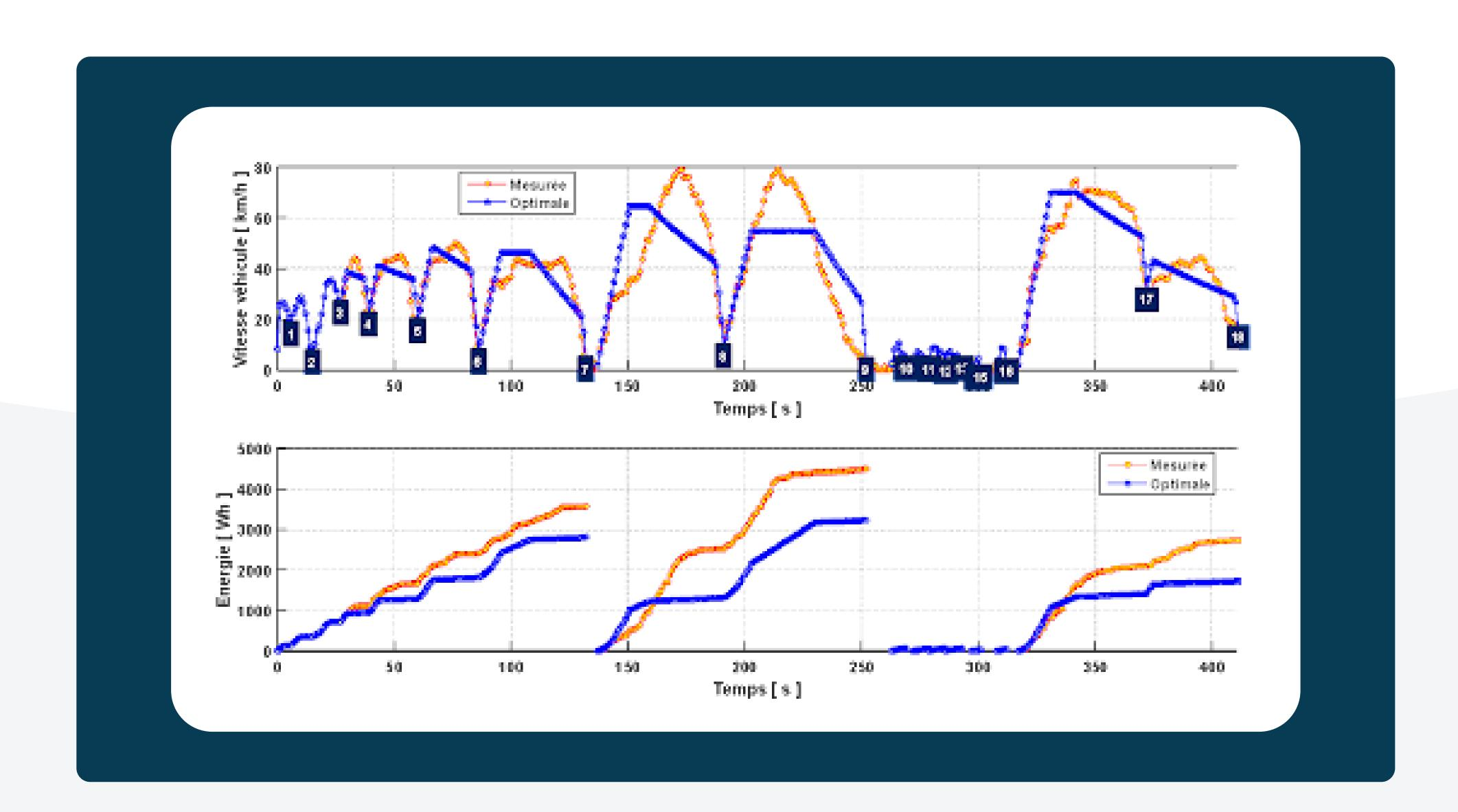
The first curve indicates that the optimal trajectory includes more full-throttle initial acceleration, a longer holding phase and later deceleration compared to the measured trajectory. The second curve shows the difference between the energy consumption measured and the optimal consumption. The following table indicates maximum possible energy savings:
