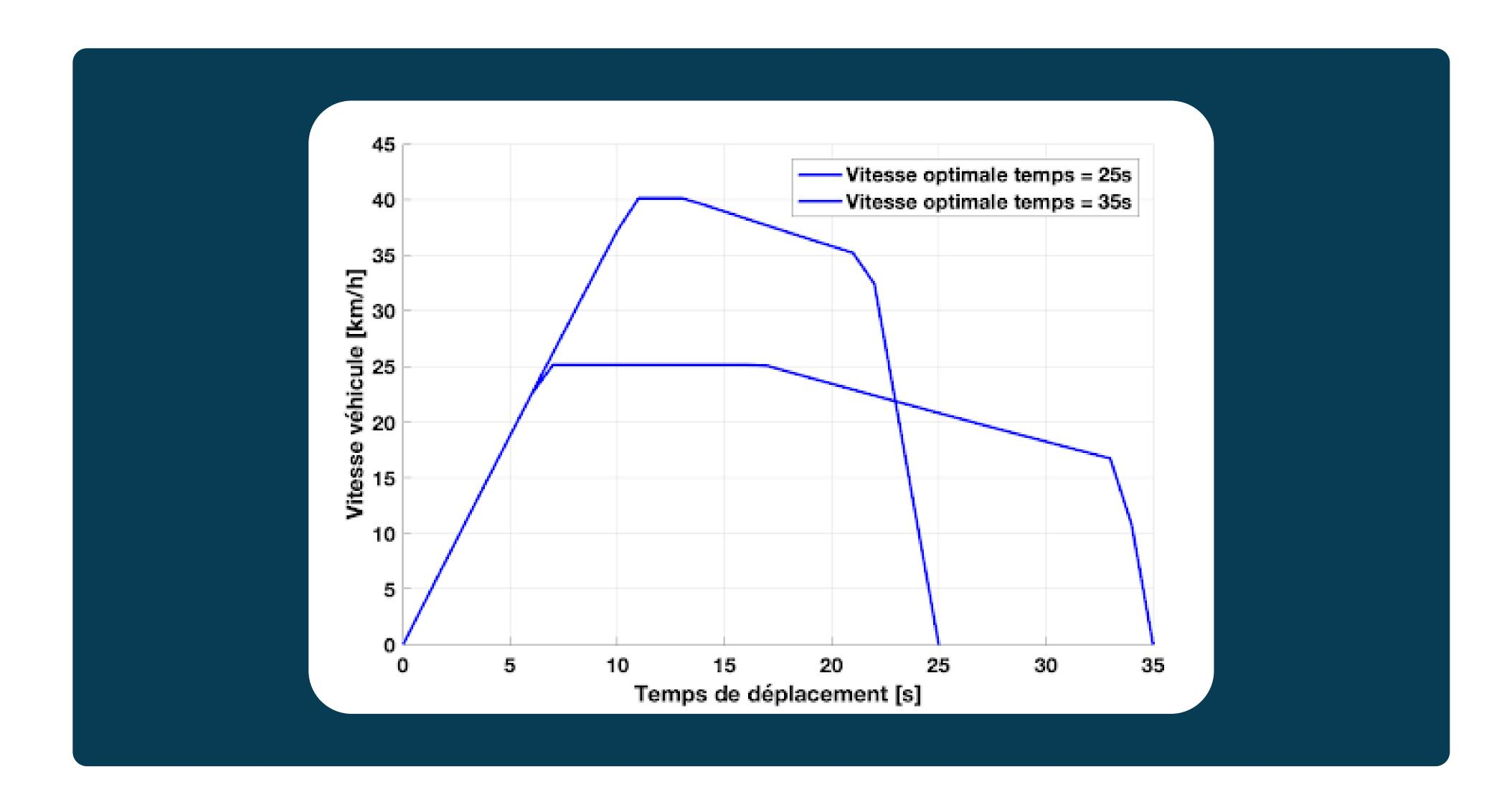
The result is very clear: the optimum speed trajectory to be adopted in order to minimise a vehicle's consumption consists of a fairly full-throttle first acceleration phase, followed by a constant speed phase, a deceleration phase (corresponding to a foot lift, when the engine is no longer producing torque) and then decisive braking.
