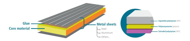
Sandwich panels consist of a core material of varying thickness, held between metal or plastic facings. They are used in a wide range of occupancies including cold storage, warehousing, the food industry, hotels, exhibition halls and clean room environments where temperature control is desirable to minimise energy loss.
