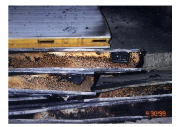
DIFFERENT RATE OF COMBUSTION OF FOAM INSULATED SANDWICH PANELS
