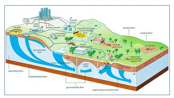
Figure 2 Diagram of the hydrological cycle showing groundwater and surface water relationships along with groundwater pollution risks<sup>21</sup>
