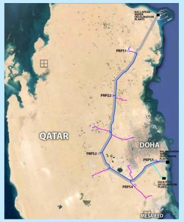
The MSR Project will construct water storage reservoirs at 5 new Primary Reservoir Pumping Stations (PRPS), which are located in the vicinity of the Qatar National Utility Corridor (QNUC). The new PRPS sites are connected to existing and future desalination plants through large diameter pipelines (Corridor Mains) that are to be constructed within the QNUC.
