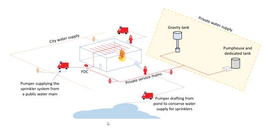
Where hose streams must be used, water should be taken from sources that do not reduce the sprinkler protection (There are no control or sectional shut off valves shown in this figure) © Franck Orset (FPO)
