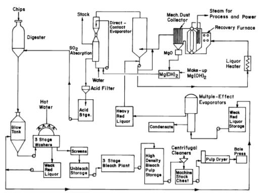
FM Global Data Sheets 7-57: Pulp and Paper Mills Fig 2 Flowchart of magnesium sulfite acid pulping and magnesium oxide recovery. Posted and reprinted with permission of FM Global. ©2010 Factory Mutual Insurance Company. All rights reserved.
