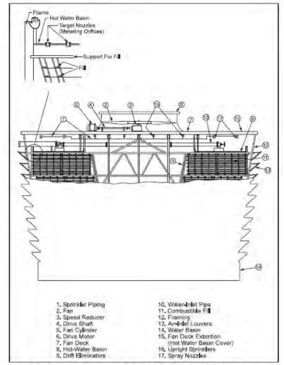
Fig. 4. Typical cross section of a crossilow induded-draft cooling tower (covered hot water basin)
