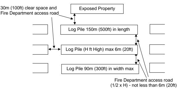
Fire lanes for access across each end, providing a clear space of at least 30m (100ft) to adjacent pile rows or other exposed property, should be provided. Where practical, greater widths are desirable to minimize the effects of radiated heat, particularly in high piled yards. Separation from main buildings should be at least 30m (100ft). See diagram below:
