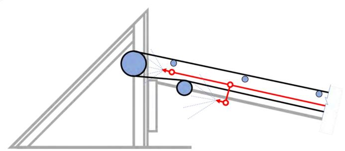
Elevation of typical end roller protection (as per NFPA 15)
