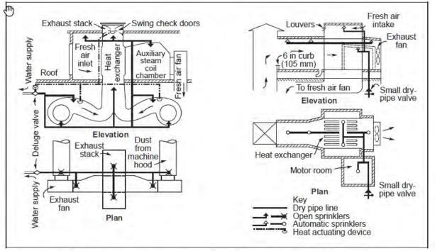
Fig. 5. Typical paper machine economizers. Suggested arragements for automatic sprinklers.
