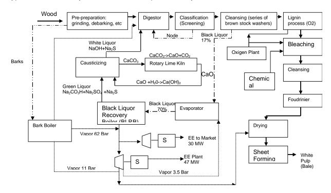
Typical Kraft Recovery Process Unit with liquor recovery and reuse.
