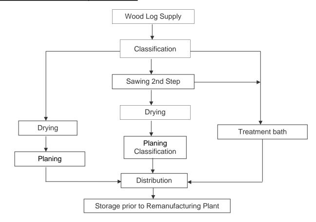
Simplified Process Block Diagram - Wood Processing Plant:
