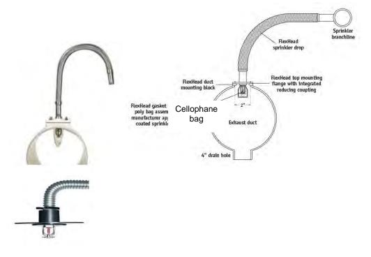
Fig. 2 - Examples of flexible sprinkler connections Posted and reprinted with permission of FM Global. ©2016-2017 Factory Mutual Insurance Company. All rights reserved.
