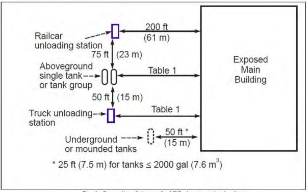
Fig. 1. Separation distances for LPG storage and unloading
