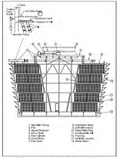
Fig. 2. Typical cross section of a crossflow induced-draft cooling lower (open hol water basin)
