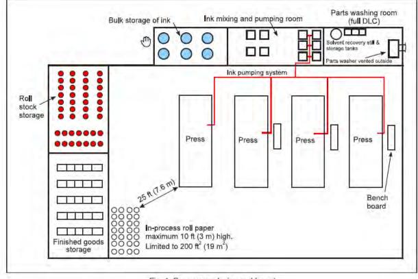
Fig. 1. Press room design and layout
