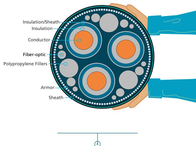
FIGURE 3: A TYPICAL CROSS-SECTION OF SUBSEA CABLE
