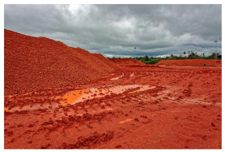
Alumina refinery "red mud" dry stacking.
