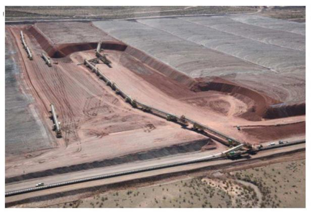
Fig 11. Self-contained movable spreader/stacker
