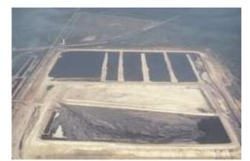
Fig 2 (a) Wet stack with single location discharge
