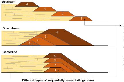
Starter dyke: 1 The dam design terms, upstream, downstream and centerline, indicate the direction in which the embankment crest moves in relation to the starter dyke at the base of the embankment wall.
