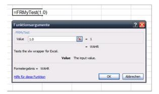
Figure 5.1: Screenshot showing the Microsoft Office Excel Function Wizard with the exemplary C++ function that was exposed to Excel via the use of xlw.
