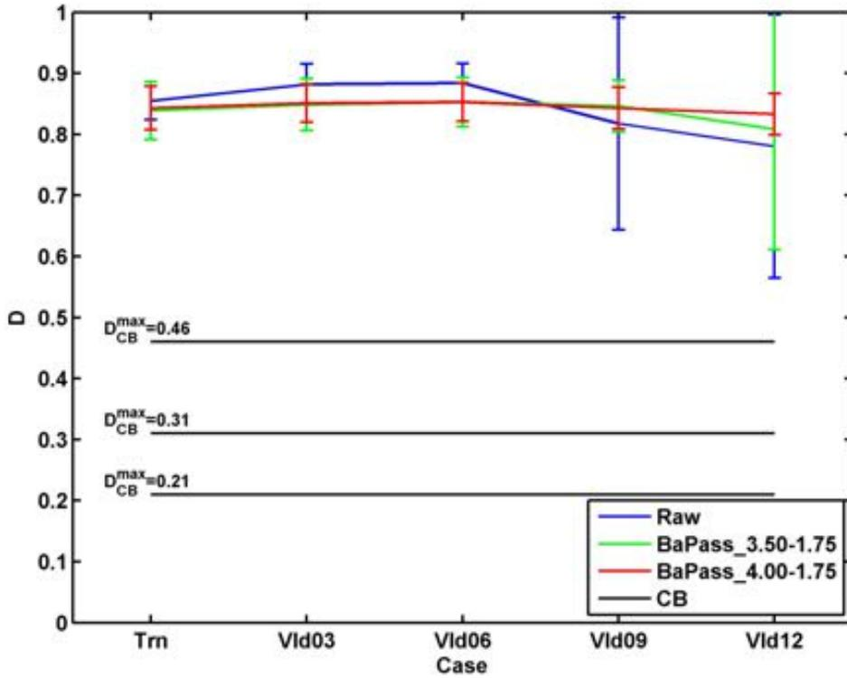
Figure 13.  $D$  scores (mean  $\pm$  2 standard deviations) for the raw data (blue line) and two optimal band-pass filtered datasets. One frequency band is from 10-3.5 to 10-1.75 Hz (green line), and the other from 10-4.0 to 10-1.75 Hz (red line). The training phase is from the onset time of each station up to 2015/03/31 (denoted as Trn in the x-axis). The validation phases are 3, 6, 9, and 12 months following the training phase (denoted as Vld03, Vld06, Vld09, and Vld12, respectively).
