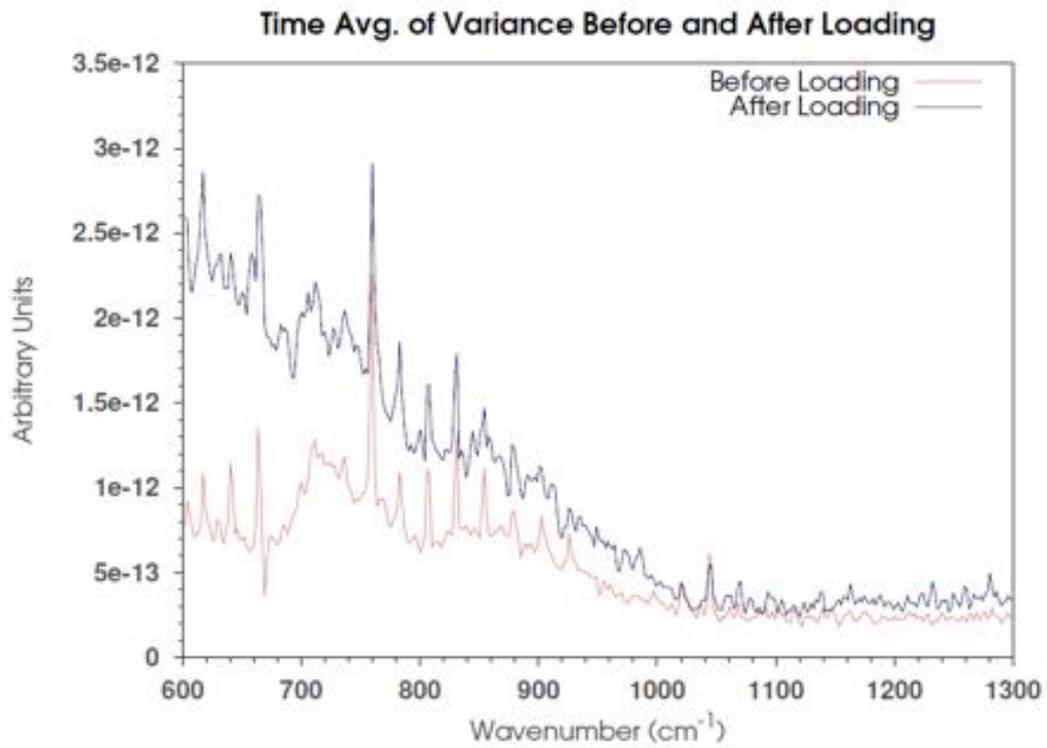
**Figure 4.** Red Granite in hydraulic press. Emission activity (average variance) versus frequency. Note the sharp, evenly spaced lines at 760, 783, 807, 831, 854, 878, 902, and 926 cm<sup>-1</sup>.
