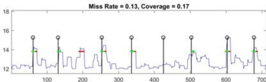
**Figure 7.** Characteristic function (blue curve) together with the tram arrival (vertical lines). The horizontal lines represent used the successful (green) and false (red) alarms obtained by thresholding at 13.8.
