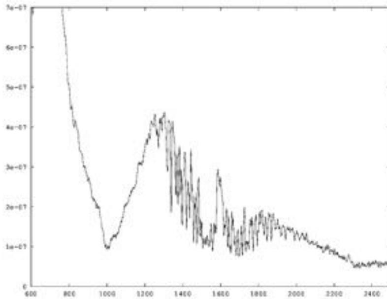
**Figure 16:** This image, from 6:40, shows the peak of TIR activity associated with a fracture event, distinct from the earlier TIR events. Note the increased presence of water lines. (spectral variance as a function of frequency)
