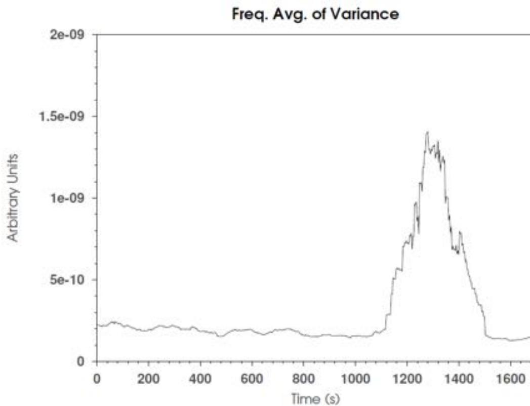
**Figure 2.** Red Granite in hydraulic press. Average spectral variance versus time, calculated in a 30-sample sliding window. The rock was eventually pulverized by the press, leading to high levels of TIR activity.
