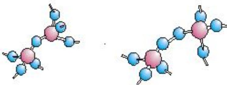
**Figure 1:** Schematic representation of a common  $O_3Si-O-SiO_3$  bond (left) and a peroxy bond,  $O_3Si-OO-SiO_3$ , where  $Si^{4+}$  may be replaced by  $Al^{3+}$  etc. The pink spheres represent the  $Si^{4+}$ , while the blue spheres (which are much larger) represent the oxygen positions.
