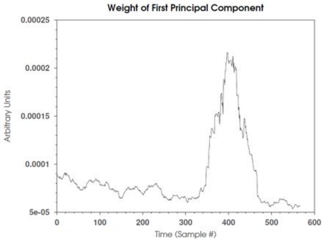
**Figure 3.** Red Granite in hydraulic press. Weight of the largest principal component versus time, calculated in a 30-sample sliding window. This is in close agreement with the fluctuation spectroscopy result shown in Figure 2.
