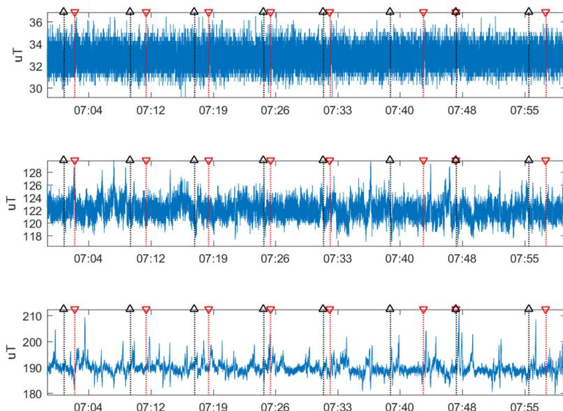
**Figure 4.** Magnetic field data on  $x$ ,  $y$  and  $z$  axes for the time interval from 8AM to 9AM overlaid with tram arrival times shown as triangles. Black: positive  $x$ -axis direction, red: negative  $x$ -axis direction.
