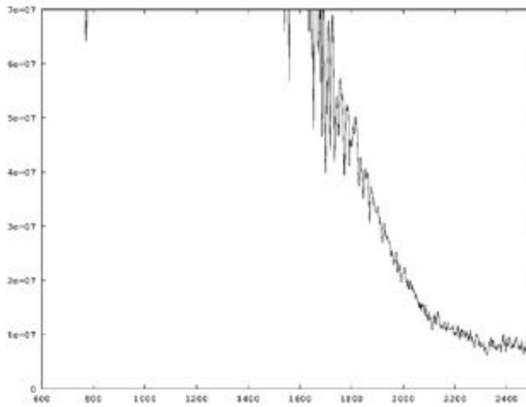
**Figure 20:** This image from the end of the 8-hour experiment shows continued TIR activity, mostly off the scale of the graph, from the fracture that destroyed the rock. (spectral variance as a function of frequency)
