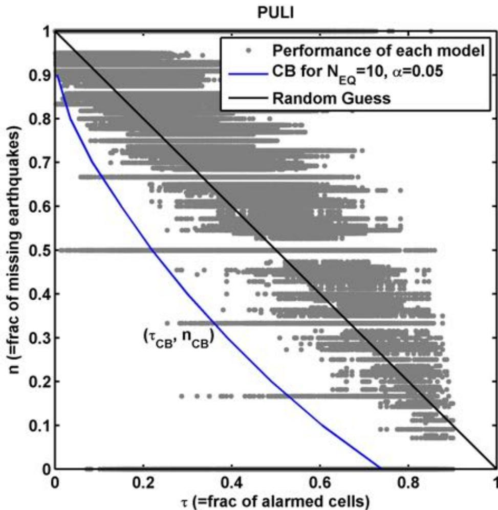
Figure 9. Molchan error diagram of the PULI station (gray dots) for the training datasets from its onset to 2015/03/31 with a confidence bound (blue line). This bound is defined at significance level  $\alpha=0.05$ , and the number of target events  $N_{EQ}=10$ . The black diagonal line stands for a random guess.
