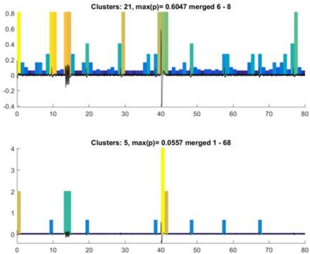
**Figure 6.** Synthetic signal overlaid with colored regions depicting individual segments. The height of the segments is proportional to their SNR score. Segments are iteratively merged together depending on the similarity of their statistical similarity.
