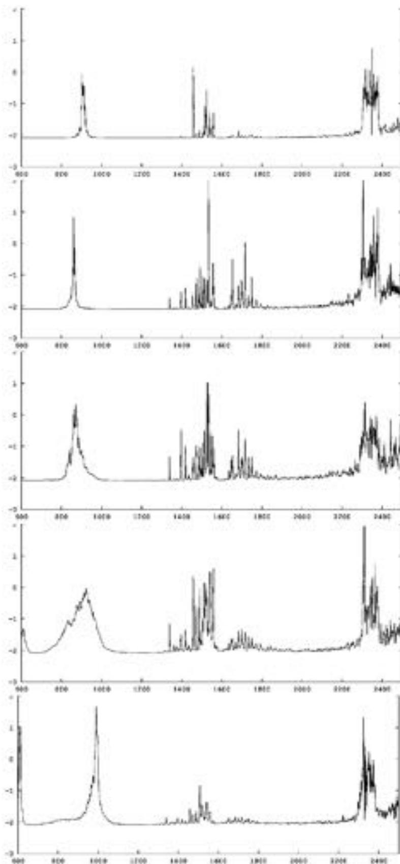
**Figure 21:** These plots show changes in spectral kurtosis (horizontal axis: frequency). In the first image, a dynamic peak can be seen just around  $900\text{-}950\text{cm}^{-1}$ . In the second, The dynamic peak has drifted below  $900\text{cm}^{-1}$ . In the third, the peak grows and changes shape. The fourth shows the continued evolution of this peak. In the last figure, the peak seems to hit an upper cutoff around  $1000\text{cm}^{-1}$ .
