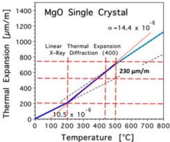
**Figure 4a:** Thermal expansion of nominally 99.99% pure single crystal MgO up to 800°C, using the fourth order of the (100) x-ray diffraction line.
