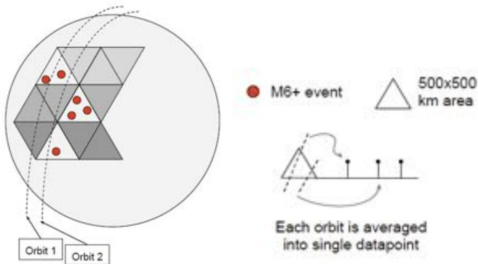
**Figure 1:** Triangular tessellation of the Earth's surface, with occurring large events (here, larger than  $M=6$ , red full circles) and two orbits corresponding to the trajectory of the satellite on the same day. The bottom right sketch shows that all measurement points on the same day over the same triangle are averaged out to get a daily measure.
