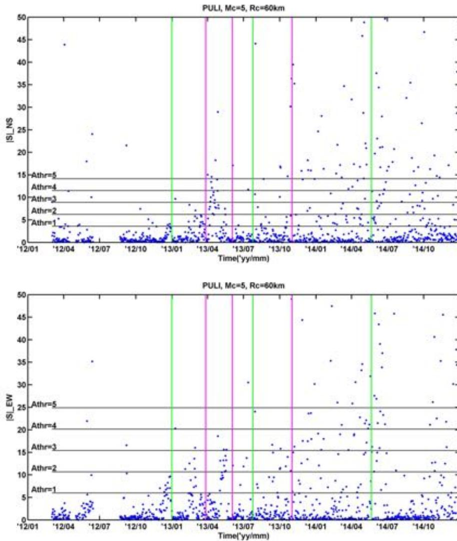
Figure 4. Time series of the absolute values of the skewness (blue dots) for the N- and E-components for the PULI station and their upper thresholds corresponding to different Athr (black lines). The green and magenta lines correspond to  $ML \in [5, 6)$  and  $ML \geq 6$  events, respectively. The distances from those events to the PULI station are smaller than or equal to 60 km.
