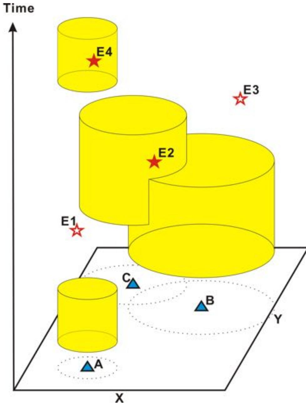
Figure 10. Schematic diagram of a joint stations method of the GEMSTIP algorithm. For example, event E2 is missed for a single station method at station B, while it is a hit considering a joint stations method using stations B and C.
