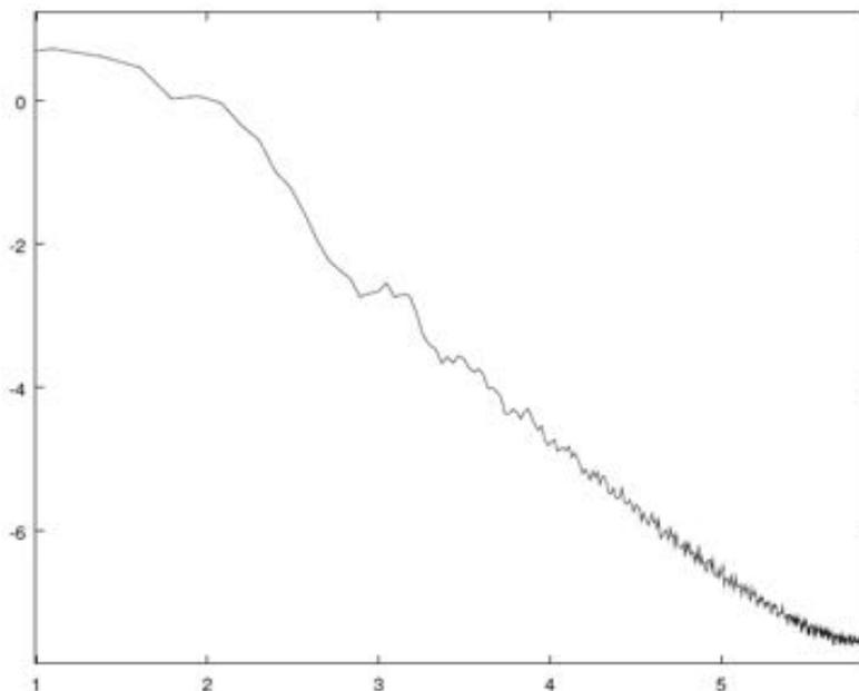
**Figure 7.** This shows log-frequency (horizontal) vs. log-amplitude (vertical) for the spectrum of the entire Bustar experiment. The slope of the line, corresponding to the critical exponent of the power law, is between -1 and -2, indicating that pink noise dominates the process.
