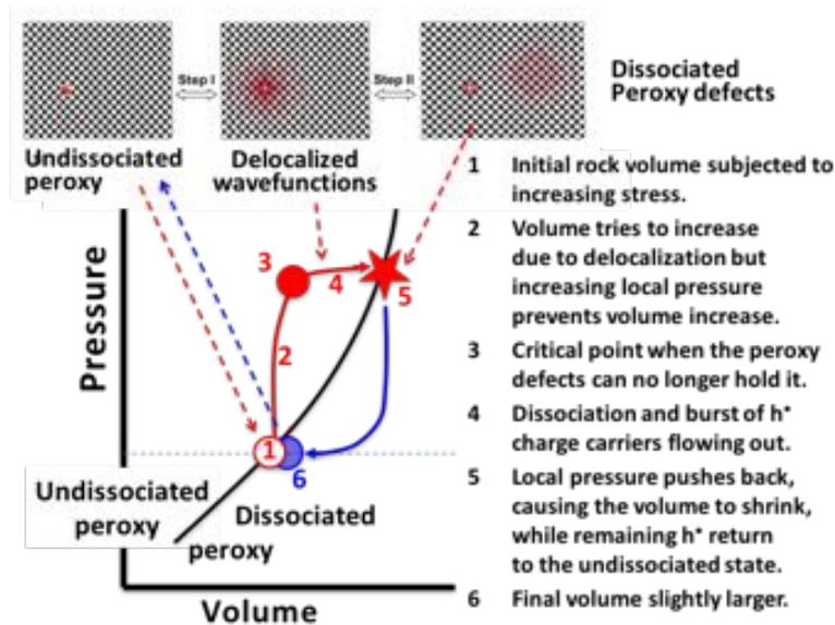
**Figure 5:** Projection of the break-up of peroxy defects onto the P–V plane. The black solid line marks the phase boundary between the fully undissociated and the fully dissociated peroxy states. 1–3 mark the pressure change due to the volume increase during the delocalization of the peroxy wave functions; 4–6 mark the volume instability during the break up (ratchet) of peroxy bonds and outburst of positive holes.
