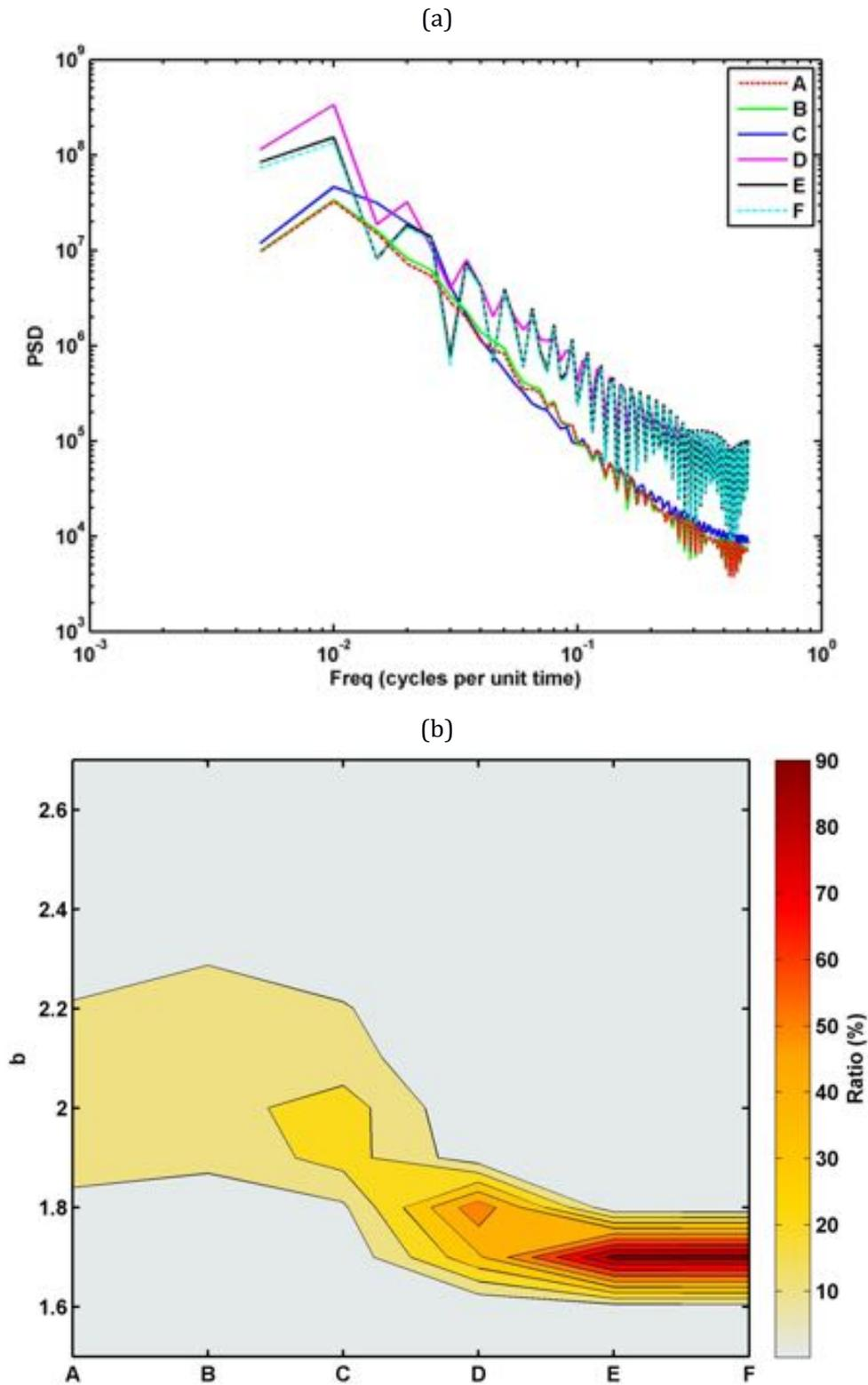
Figure 6. (a) Average of power spectrum densities (PSDs) of the 305 non-overlapping segments, whose length is 131 time units per segment. (b) Statistical distributions of power-law exponents ( $b$  value) of power-law fitting in the 305 PSDs.
