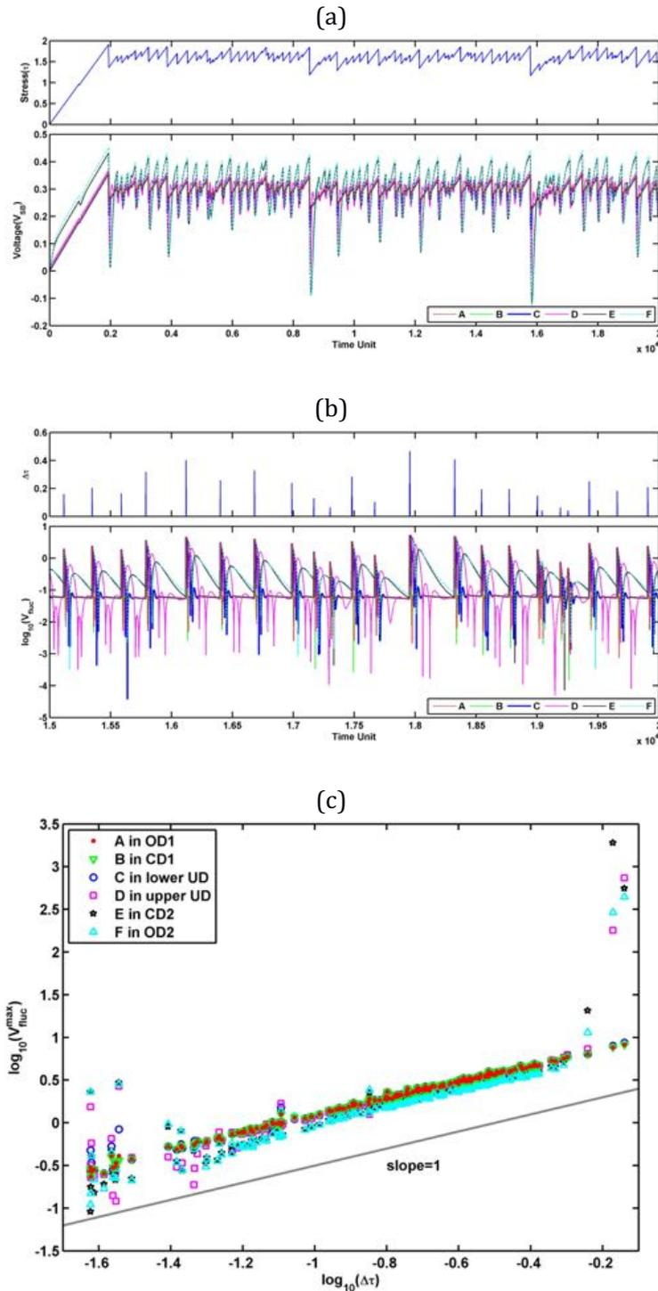
Figure 3. In the single-block model, (a) time series of stress ( $\tau$ ) and its block voltage ( $V_{SB}$ ) for sets A to F. (b) Time series of stress drop ( $\Delta\tau$ ) and relative voltage fluctuation ( $V_{fluc}$ ) for sets A to F. (c) Scatter plot of the stress drop of an event and its corresponding maximal voltage fluctuation in a log-log scale. The gray line with slope=1 is plotted as reference.
