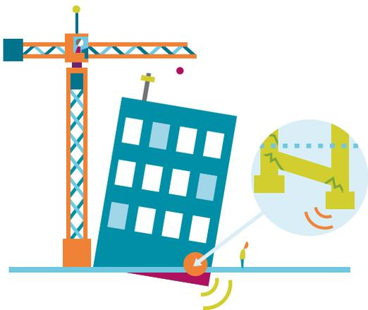
Foundation failure causing building settlement: possible causes include geotechnical or foundation design errors.
